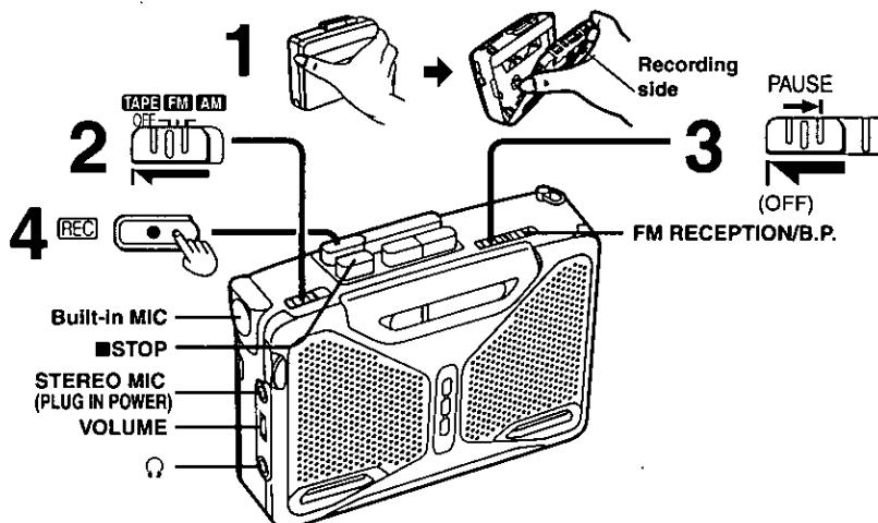
STEREO MIC [Plug type : 3.5mm (1/8 in.) Stereo]
